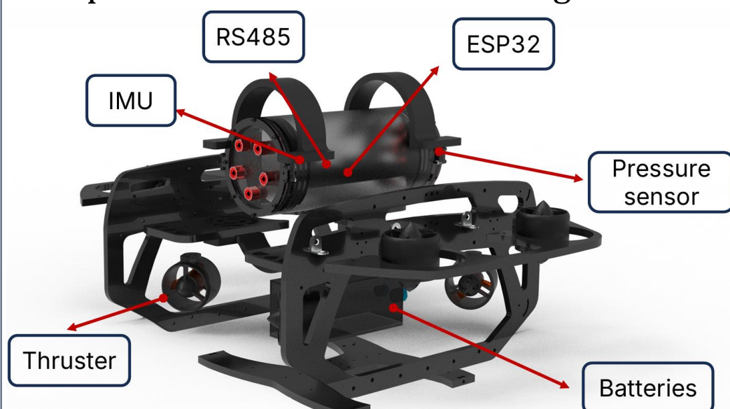
Fig. 3: Exploded view of our EasyUUV hardware platform.
