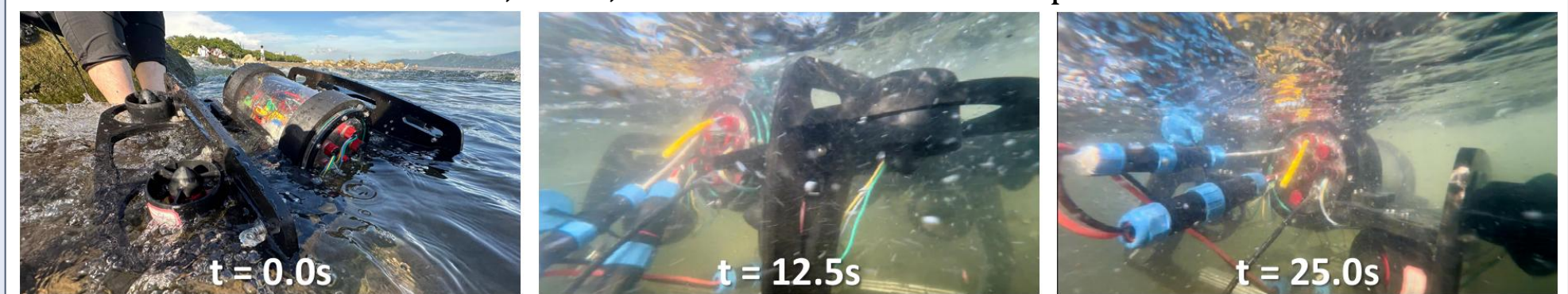
Fig. 7: Snapshots of EasyUUV operating in real ocean conditions at t = 0.0s, 12.5s, and 25.0s in sea trials
