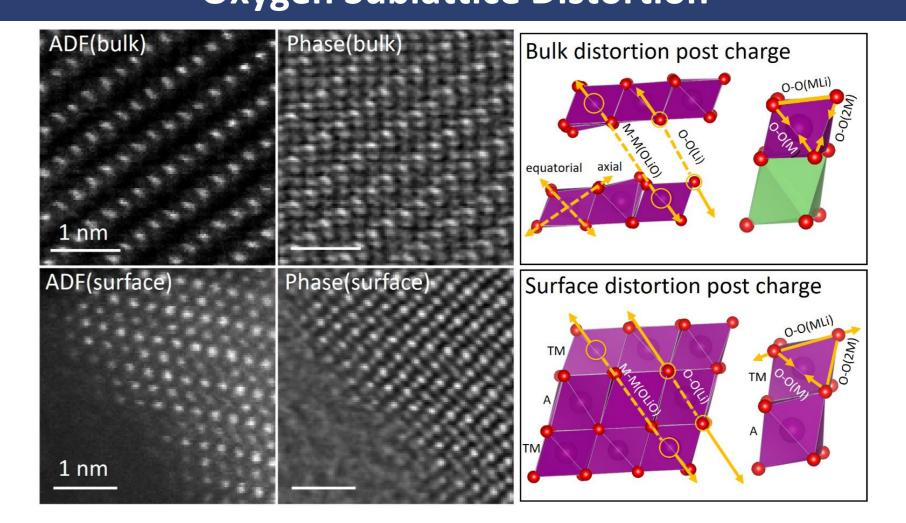
Imaging of oxygen sublattice and measuring  $[TMO_6]$  octahedral distortion with pico-meter precision from bulk and surface.
