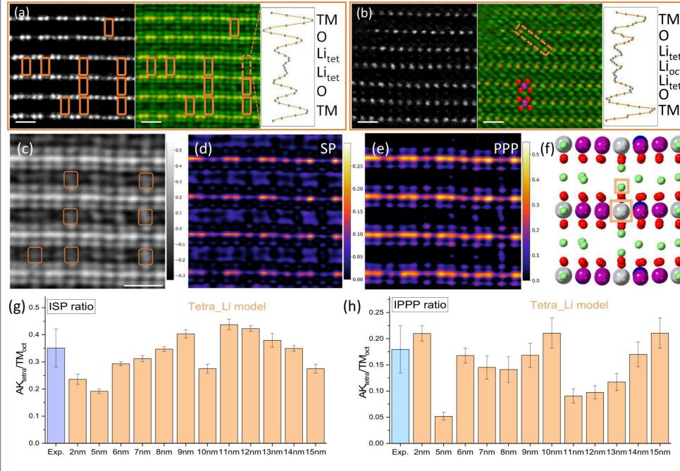
Ptychographic phase quantification demonstrates lithium diffusion from TM-layer to alkali layer through the tetrahedral sites of  $\rm Li_{1.2}[Ni_{0.13}Mn_{0.54}Co_{0.13}]O_2$ .
