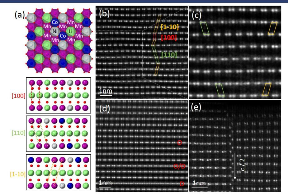
ADF imaging of  $Li_{1.2}[Ni_{0.13}Mn_{0.54}Co_{0.13}]O_2$  showing inter-layer and intra-layer stacking faults with ordered and disordered contrast.
